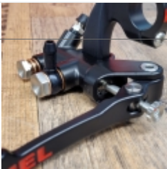
Connection to expansion tank 90° Banjo
