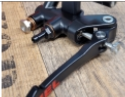
Connection to expansion tank straight
